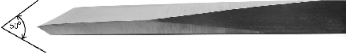
2. Negative Rake Scrapers only cut with the burr that is developed during the grinding process. The burr does not last long, about 30 to 60 seconds for M2 HSS and 2 to 3 times longer with the harder "powdered metal" steel tools, i.e. Thompson tools and others. The burr is produced on the opposite edge that is being ground.
